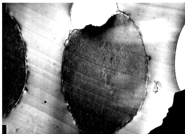
Figure 6. Horizontal cross-sectional TEM image of PS- b -PVP columns.
